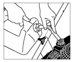
**Step 5** Fill gas tank with unleaded gasoline. Do not use leaded gasoline.
